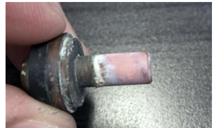
Figure 4: Piston Seized in Lime Before Installation of the Mag-O-Pure Catalyzer.
