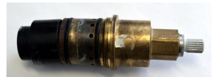
Figure 3: Defective Thermostatic Valve
